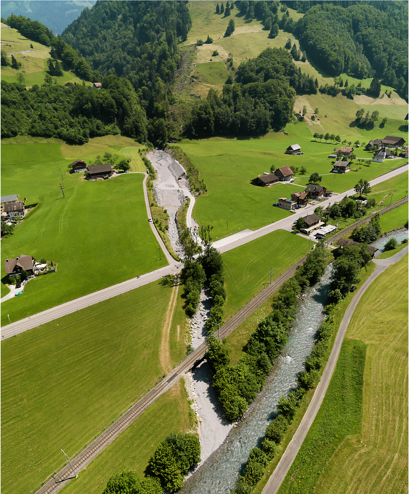
Secklisbachsammler The modified lower channel in Secklisbach
